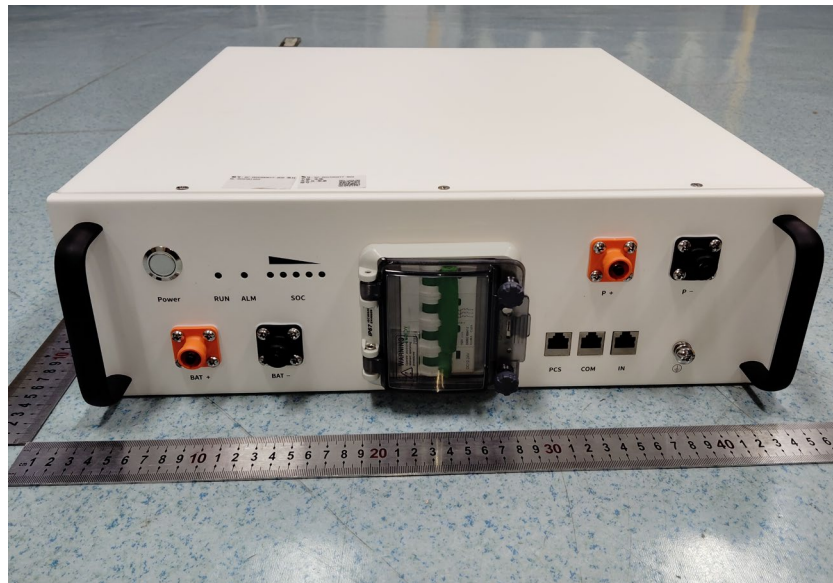
control box JRH51-PDU communication port
